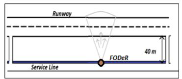
The below illustration portrays the runway and the service line(blue colored area). As shown, the FODeR is placed in the service line, from there the FODeR scans the runway as specified earlier. So by moving to and fro in the service line the runway can be scanned on the whole. Once the FOD is detected the FODeR will go to the runway using the links that connect the runway and service line.
